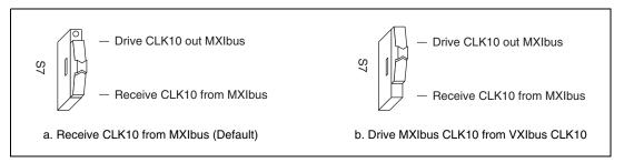
Figure 3-7. Receiving or Driving MXIbus CLK10
